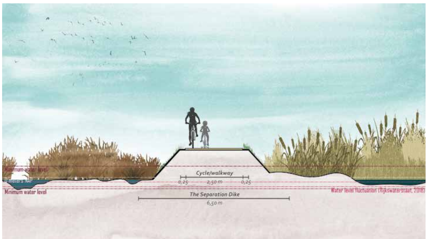
Figure 76: Detailed separating dike between fresh and salt ecotopes
