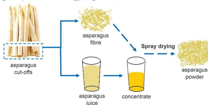
**Figure 2:** Split-stream processing strategy of white asparagus waste bottom parts. Figure reproduced with permission from [4].
