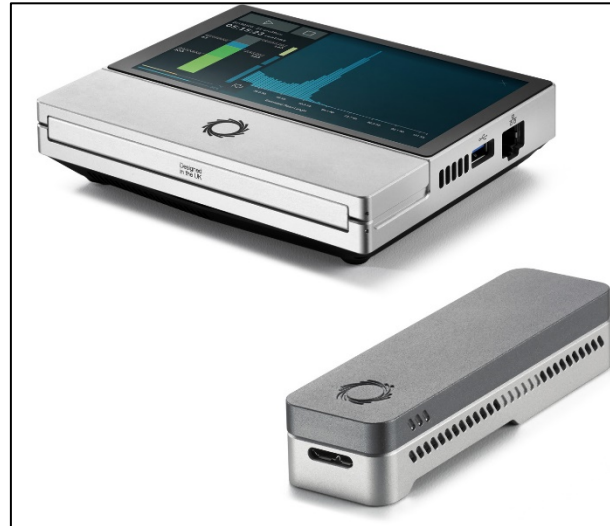
Figure 2. Bottom: MinION Mk1B which requires a laptop for on-site DNA sequencing. Top: MinION Mk1C which can perform DNA sequencing fully autonomous (nanoporetech.com).
