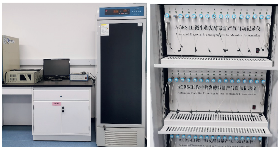
Figure S4.1. The in vitro gas production machine with Automated Gas Production Recording System.
