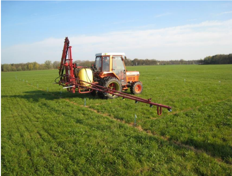
Photo 1 Field sprayer of WUR Unifarm used for application of the liquid mineral nitrogen fertiliser UAN.
