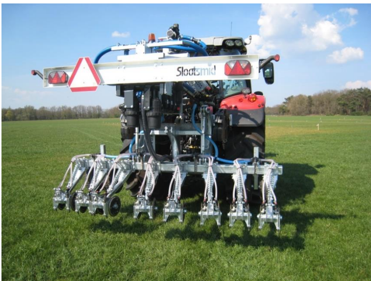
Photo 2 Injector designed for biobased fertilising products. The injector was built by Sloopsmid 29 in 2020 and was designed for use specifically in field experiments and/or fertilisation of small plots. The design aims to mitigate/minimise ammonia losses.
