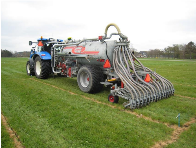
Photo 3 Injector of WUR Unifarm which was designed for the application of animal slurries. The injector was adjusted for application of cattle slurry on grassland with slots distanced at 25 cm in this photograph.
