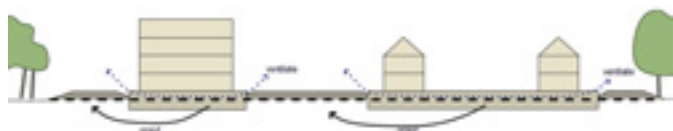
Fig. 18: Parking garages under buildings, half-deepened, creating more green open space, the excavated soil is used for raising the ground level to better fit in the landscape; source: Wurck
