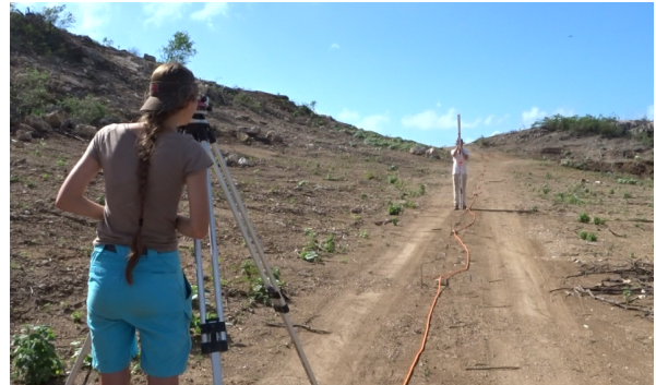
Figure 11: Land surveying at Piscadera bay. The surveyor looks through the optical level and notes down the height observed of the measuring stick.
