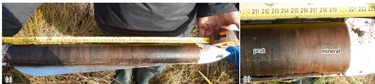
Fig. 4. Photograph of core S17 taken directly after collecting the core in the field, (a) overview photo (bottom at the right), (b) detail of the mineral-to-peat transition.
