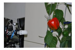
**Figure 3.** Camera mounted on robotic arm acquiring images of red sweet pepper mounted on a pepper plant.
