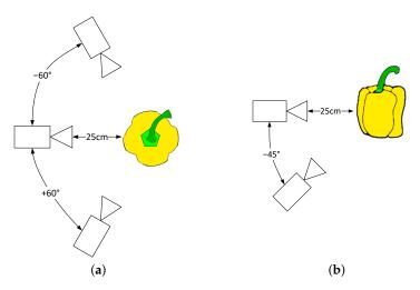
**Figure 4.** The six viewpoints are combinations of 3 different azimuth (**a**) and 2 different tilt (**b**) angles. Adapted from Harel et al. [31].
