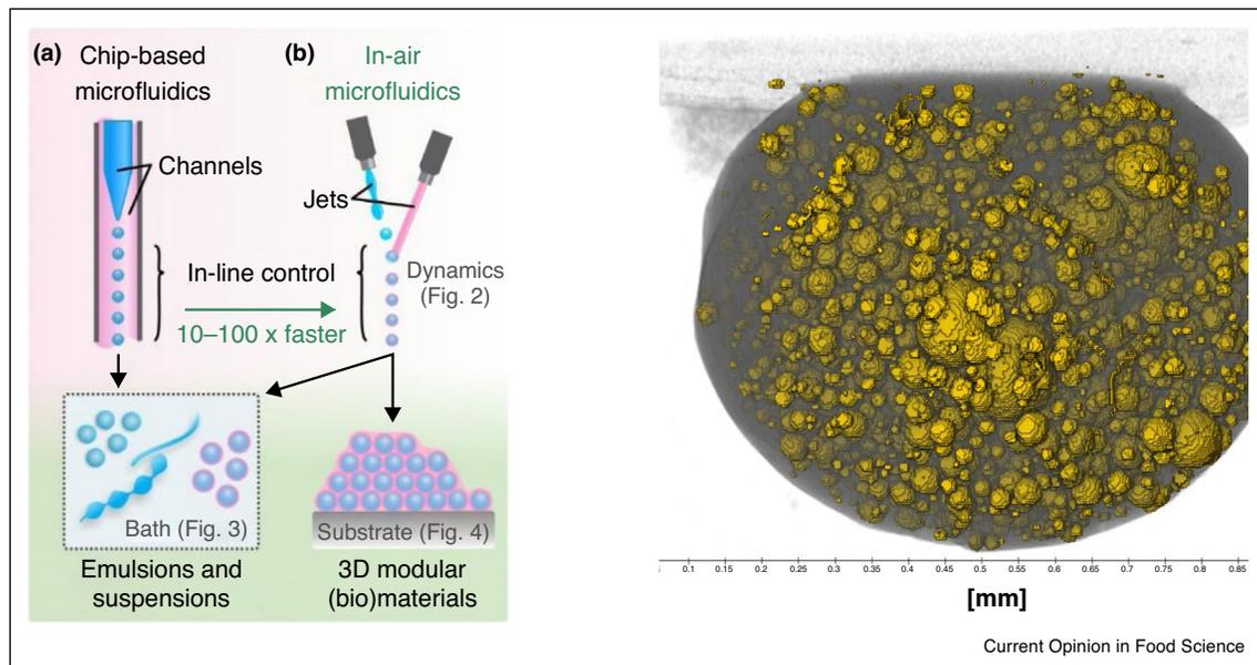
Illustration of (a) classic emulsion preparation with a microfluidic device followed by solidification in a bath, (b) in-air microfluidics in which both steps are combined [40\*]. (c) Alginate microgel capsules with multiple oil droplets prepared with a gas-assisted nozzle [41].
