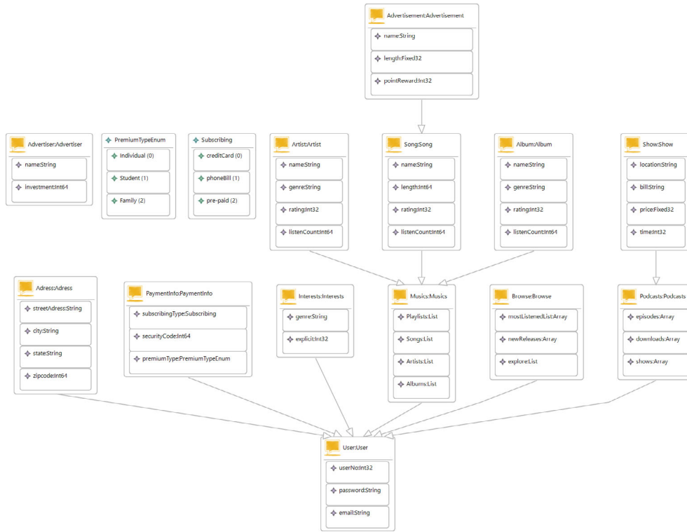
FIGURE 5 Microservice data exchange model for the case study—Object classes, attributes, and their data types
