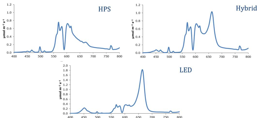
Figure 1. Spectra of the light in the three treatments. On the x-axis the wavelength in nm.
