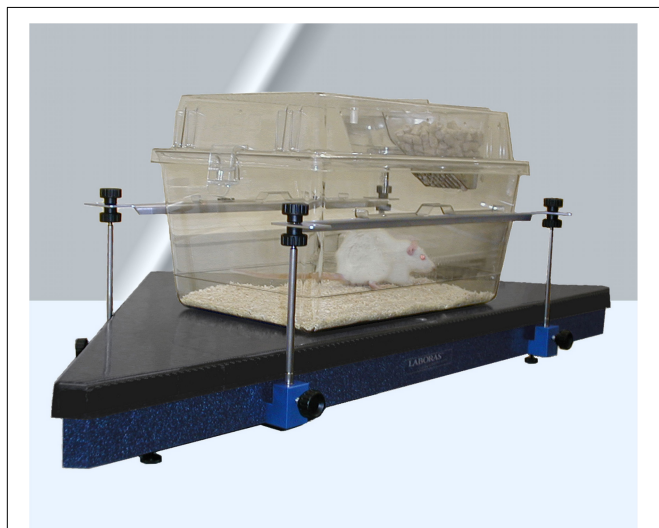
FIGURE 4 | The measurement platform LABORAS turns animal's movement into electrical signals to analyze an extended set of rodent behavioral patterns (Metris b.v.).
