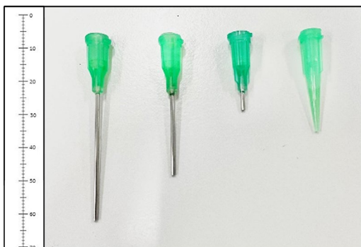
Figure 4.1. Nozzle tips used for extrusion and printing. Nozzles from left to right: long straight nozzle (metal part 38.1 mm), medium straight nozzle (metal part 25.4 mm), short straight nozzle (metal part 6.35 mm) and tapered nozzle (31.2 mm). All nozzles have an outlet diameter of 0.84 mm.
