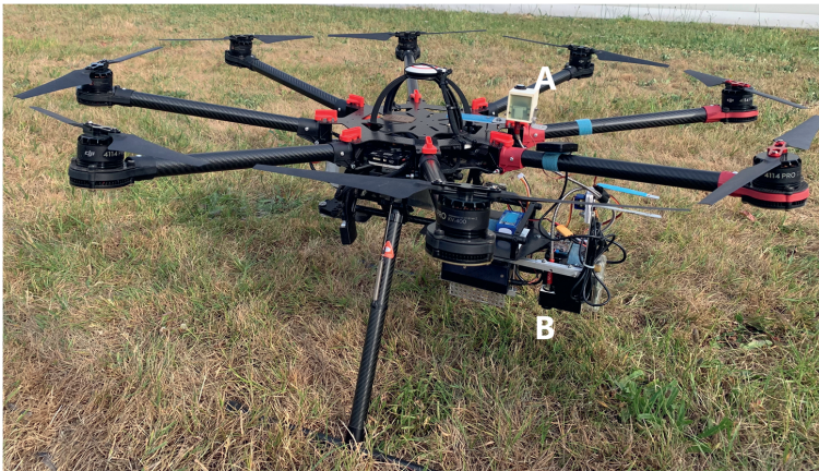
Figure 2.5. DJI S1000 octocopter UAV platform with the FluorSpec mounted. “A” refers to the FluorSpec irradiance sensor and “B” refers to the radiance sensor.
