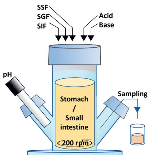
Figure 5.1: Schematic representation of SIM *in vitro* model of the infant gastrointestinal tract. SSF = simulated saliva fluid, SGF = simulated gastric fluid, SIF = Simulated intestinal fluid.
