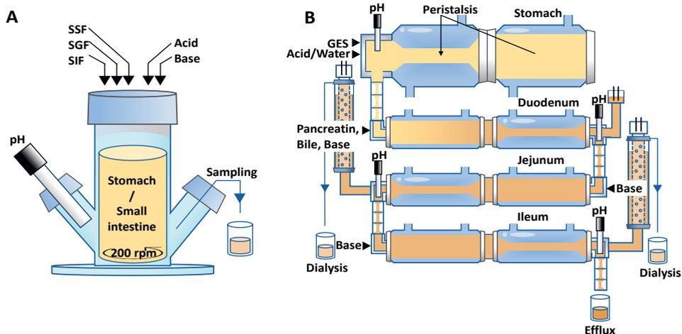
Figure 4.1: Schematic representation of the *in vitro* models used to simulate infant gastrointestinal conditions. A) Semi-dynamic *in vitro* model of the gastrointestinal tract (SIM). B) Dynamic model of the gastrointestinal tract (TIM-1), adapted from [13]. SGF = simulated gastric fluid, SIF = simulated intestinal fluid, SSF = simulated saliva fluid, GES = gastric enzyme solution.
