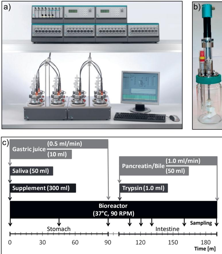
Figure 2.1: Semi-dynamic model of the gastrointestinal tract. The model consisted of A) Computer controlled parallel bioreactor system, and B) Single bioreactor with overhead agitation. C) Time schedule.
