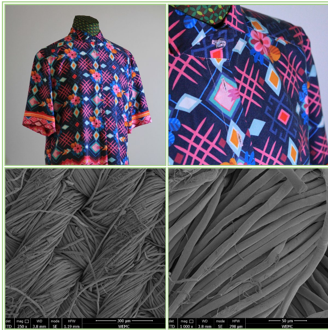
Figure 19: Example of a lyocell fabric (satin weave) composed of 100% lyocell. Garment and SEM pictures of the fabric.
