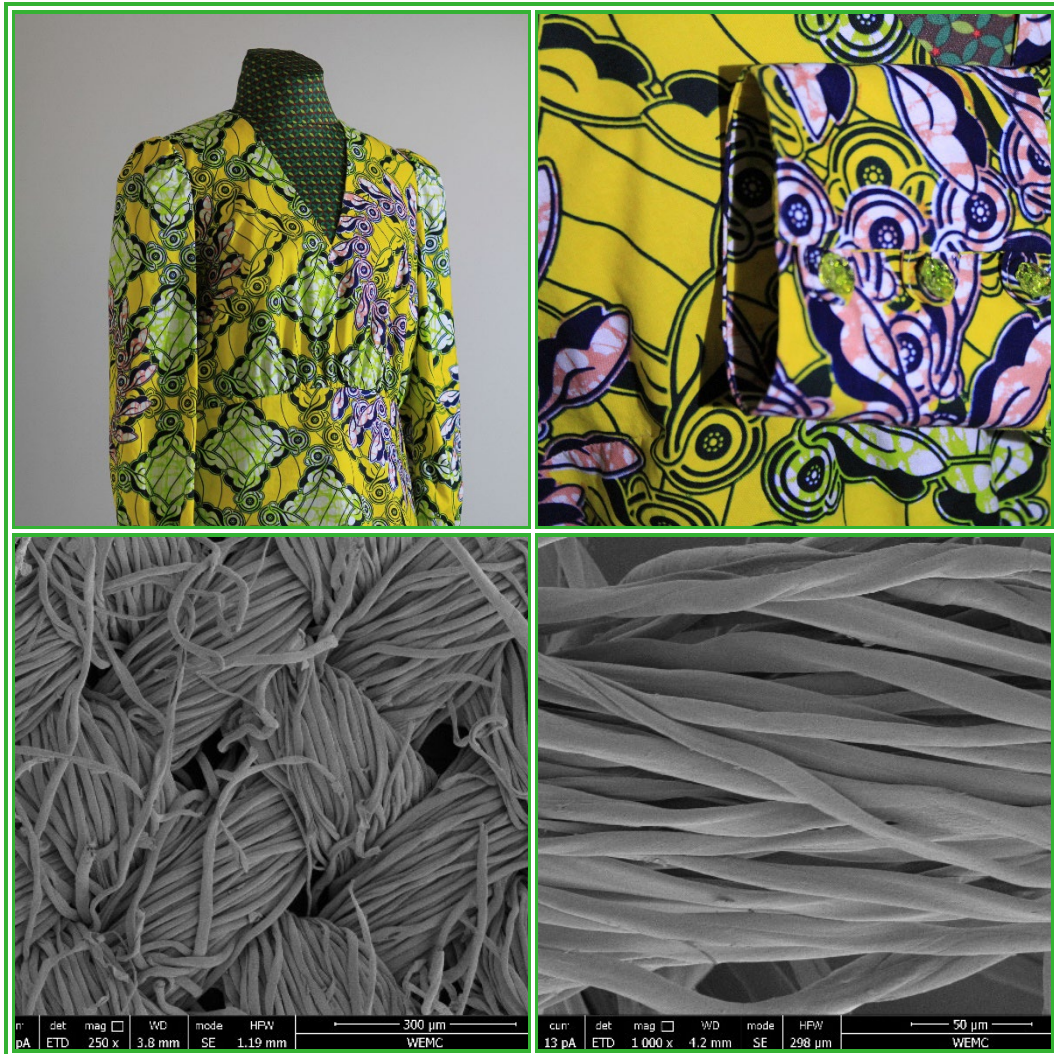
Figure 21: Example of a cotton fabric (plain weave), composed of 100% cotton. Garment and SEM pictures of the fabric.
