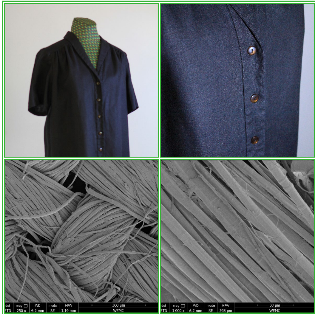
Figure 25: Example of a linen fabric (plain weave), composed of 100% linen. Garment and SEM pictures of the fabric.
