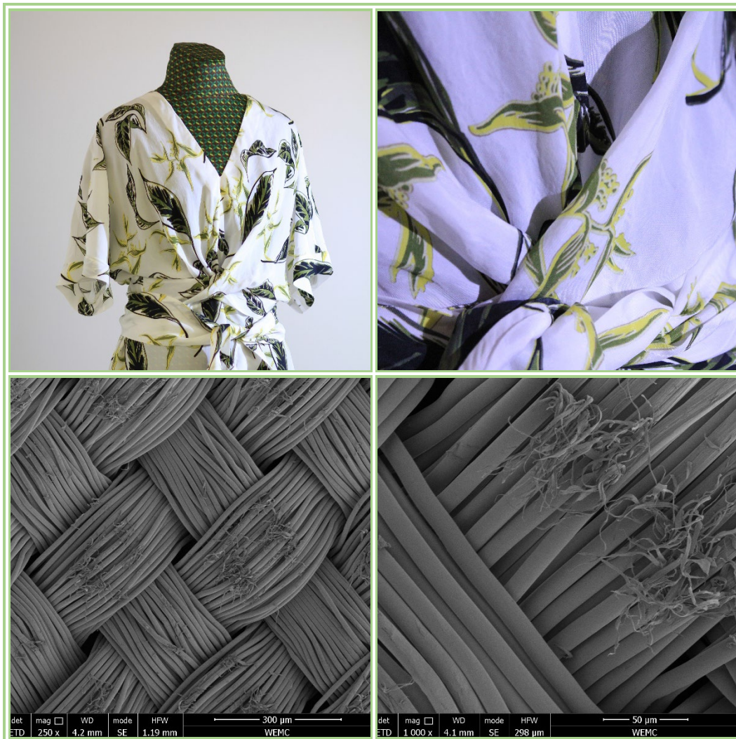
Figure 18: Example of a cupro fabric (plain weave) composed of 100% cupro. Garment and SEM pictures of the fabric.
