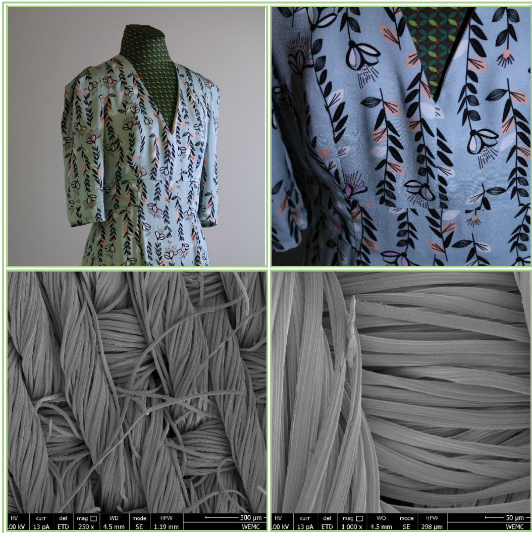
Figure 17: Example of a viscose fabric (satin weave) composed of 100% viscose. Garment and SEM pictures of the fabric.
