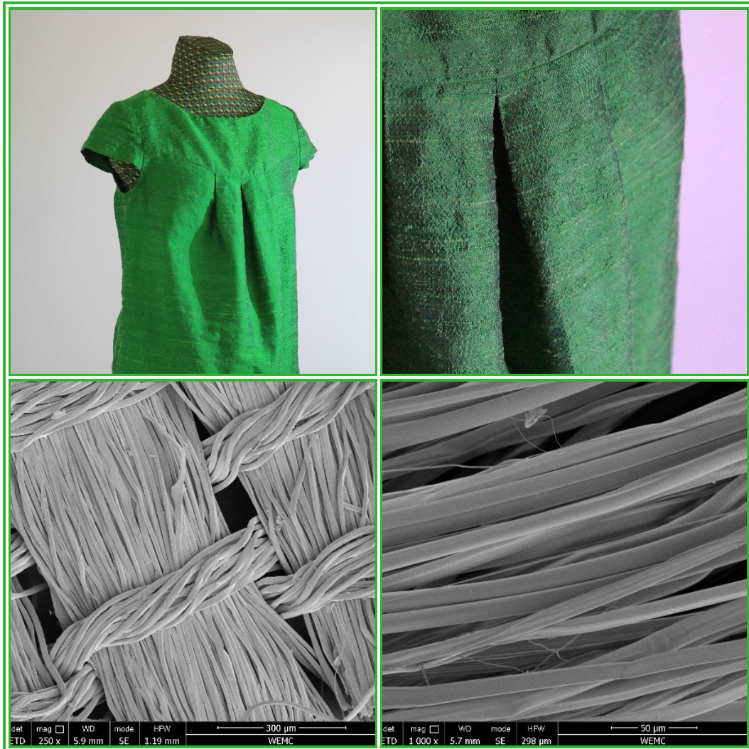
Figure 36: Example of a silk, composed of 100% silk. Garment and SEM pictures of the fabric.
