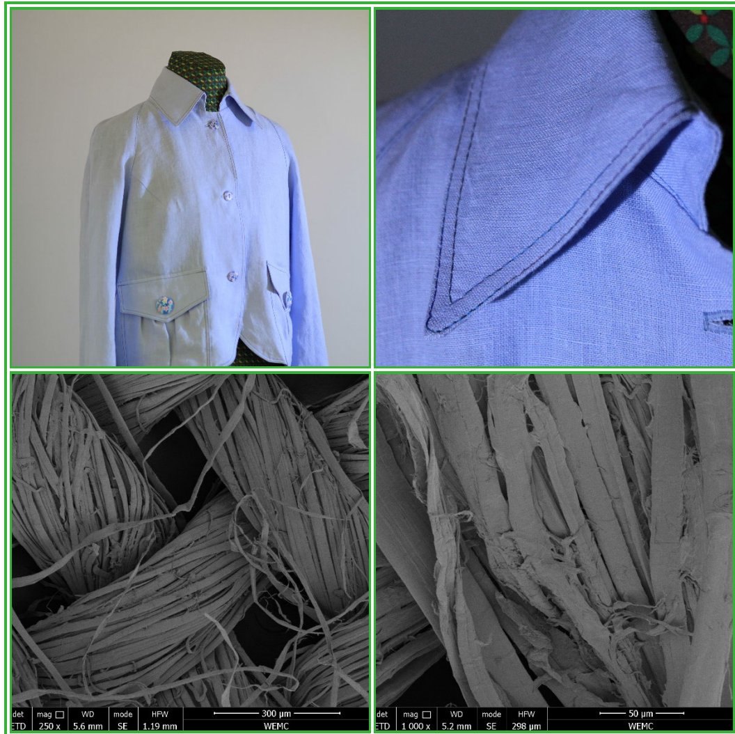
Figure 27: Example of a hemp fabric (plain weave), composed of 100% hemp. Garment SEM pictures of the fabric
