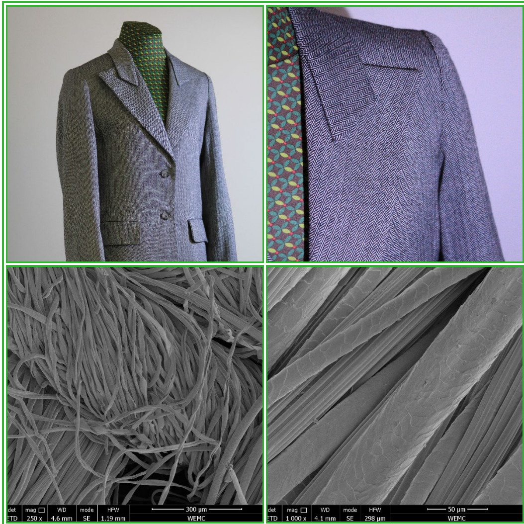
Figure 51: Example of a herringbone fabric, composed of recycled cotton, viscose, and wool. Garment and SEM-pictures of fabric.
