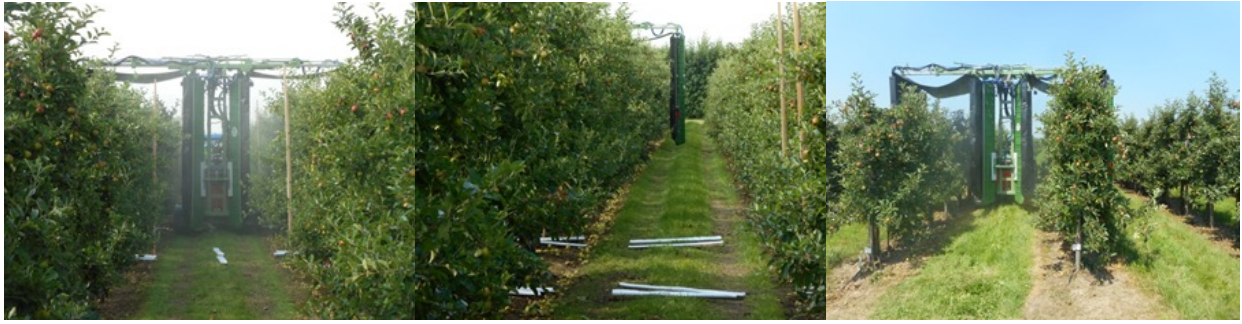
Fig. 1. Spray deposition measurements of Lochmann two-row tunnel orchard sprayer; ground deposition and spray volume in sprayer driving path (left), next path ground deposition and spray drift potential (centre), in tree deposition (right).
