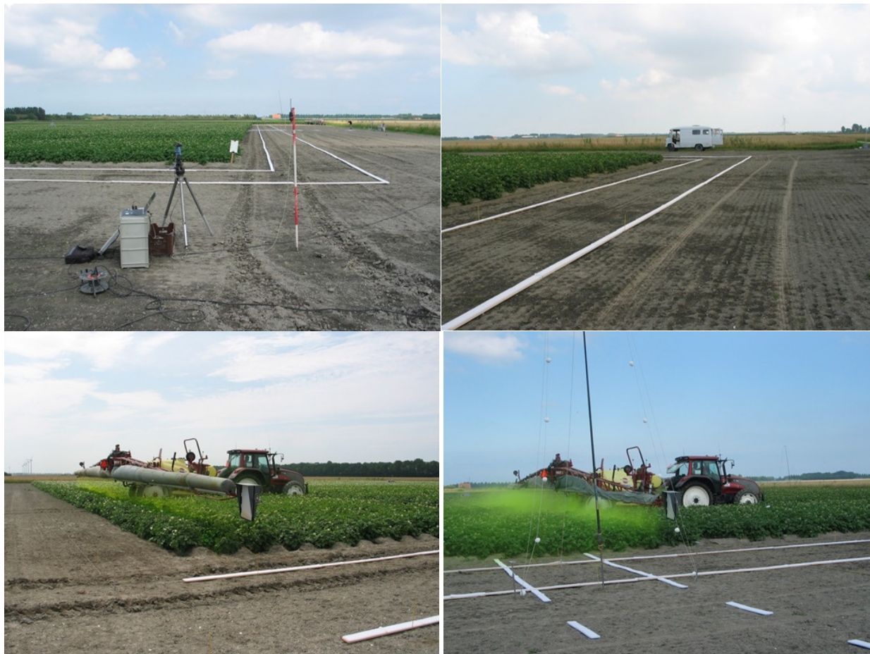
Fig. 2. Spray drift collector strips along field edge at 2 m and 5 m distance (top), with spray boom movement measuring device (top right); start of spraying swath at upwind headland field edge (bottom left) and sprayer passing the standard spray drift halfway the downwind edge of the field (bottom right).
