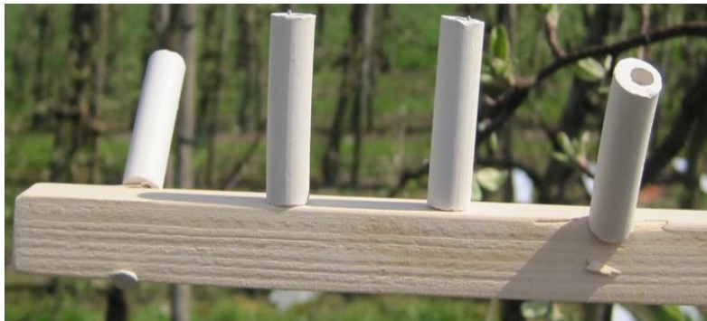
Figure 2. Clay pipes fixed to horizontal bar at three heights in the tree to mimic tree branches.
