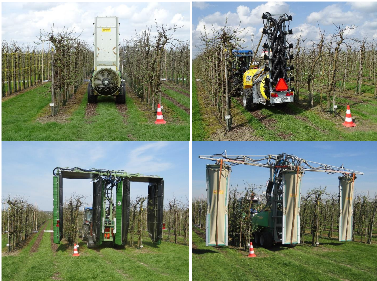
Figure 3. Sprayers used for assessing spray deposition in the early leaf stage of the apple trees: Munckhof cross-flow (top left), H.S.S. cross-flow (top right), Lochmann 2-row tunnel (bottom left), Munckhof 2-row cross-flow (bottom right).
