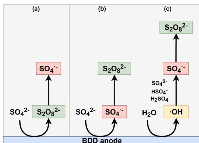
Fig. 1. Possible mechanisms of peroxydisulfate formation with BDD anode.
