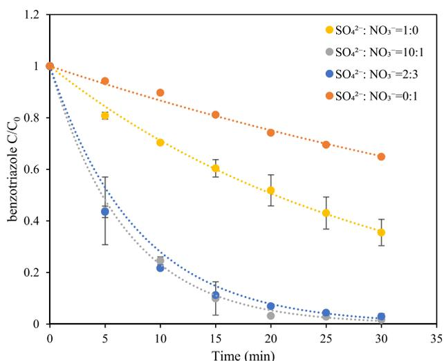
**Fig. 3.** Benzotriazole concentration changing with reaction time (min) in different  $\text{Na}_2\text{SO}_4:\text{NaNO}_3$  (SN) ratios. Experimental conditions: 10 mg/L benzotriazole, different electrolyte ratios,  $T = 25\text{--}30\text{ }^\circ\text{C}$ , applied potential = 4.3 V (vs. Ag/AgCl), conductivity = 10 mS/cm, flow rate = 580 mL/min.
