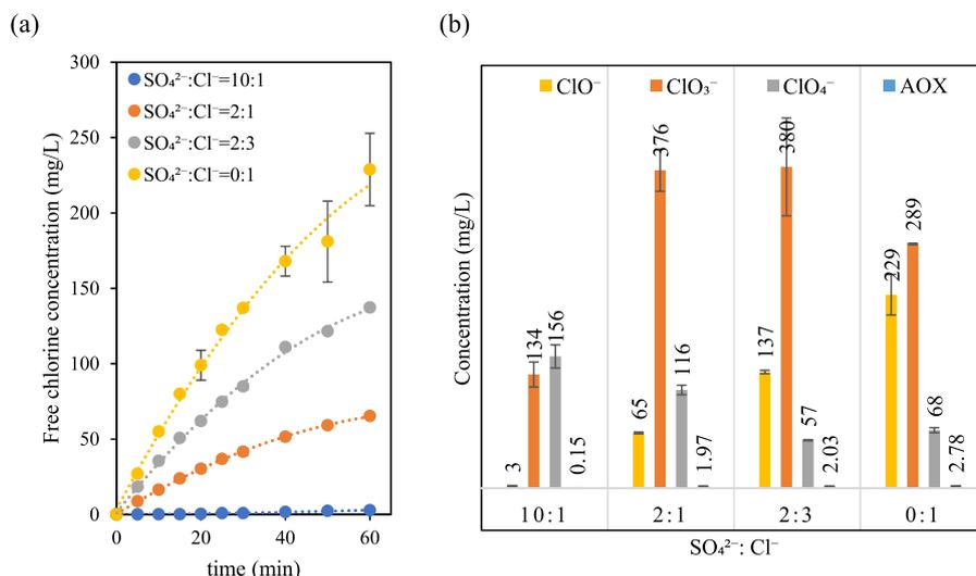
**Fig. 5.** (a) Free chlorine concentration changing with reaction time (min); (b) Free chlorine, chlorate, perchlorate and AOX concentration in different Na<sub>2</sub>SO<sub>4</sub>:NaCl (S/Cl) ratios after 60 min of treatment. Experimental conditions: 10 mg/L benzotriazole, T = 25–30 °C, applied potential = 4.3 V (vs. Ag/AgCl), conductivity = 10 mS/cm, flow rate = 580 mL/min, reaction time = 60 min.
