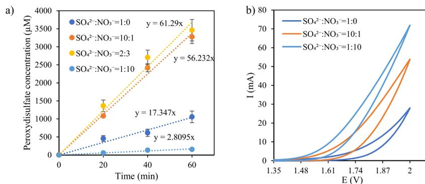
Fig. 2. (a) Peroxydisulfate concentration ( $\mu\text{M}$ ) changing with reaction time (min) in different  $\text{Na}_2\text{SO}_4:\text{NaNO}_3$  ratios. Experimental conditions:  $T = 25\text{--}30^\circ\text{C}$ , applied potential = 4.3 V (vs. Ag/AgCl), conductivity = 10 mS/cm, flow rate = 580 mL/min (b) cyclic voltammetry tests in different  $\text{Na}_2\text{SO}_4:\text{NaNO}_3$  ratios; scan rate 50 mV/s, applied potential 0.2-0 (vs. Ag/AgCl), conductivity 10 mS/cm.
