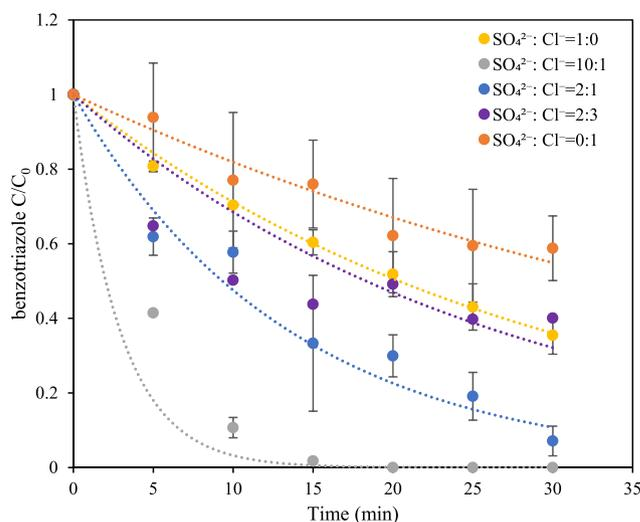
**Fig. 4.** Benzotriazole concentration changing with reaction time (min) in different  $\text{Na}_2\text{SO}_4:\text{NaCl}$  (SCL) ratios. Experimental conditions: 10 mg/L benzotriazole,  $T = 25\text{--}30\text{ }^\circ\text{C}$ , applied potential = 4.3 V (vs. Ag/AgCl), conductivity = 10 mS/cm, flow rate = 580 mL/min.
