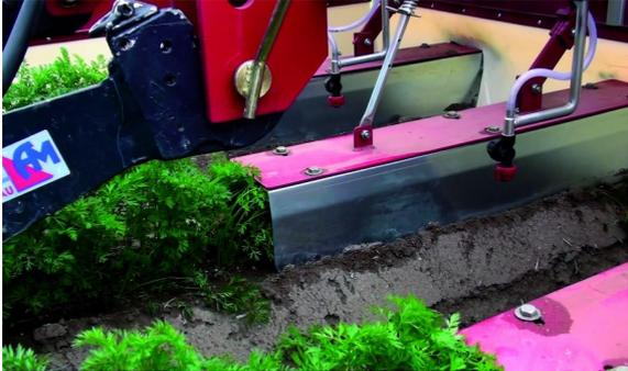
**Figure 7B** Sprayer for strip application equipped with tunnels protecting the crop during inter-row application
