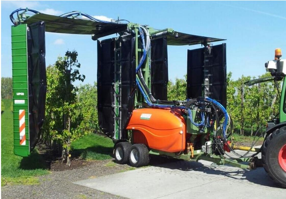
**Figure 9** Two row tunnel-sprayer with recirculation-system
