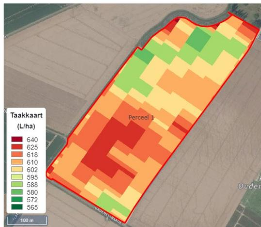
**Figure 3C** Task-map (taking into account sprayer dimensions) converted to tank-mix in litres per ha
