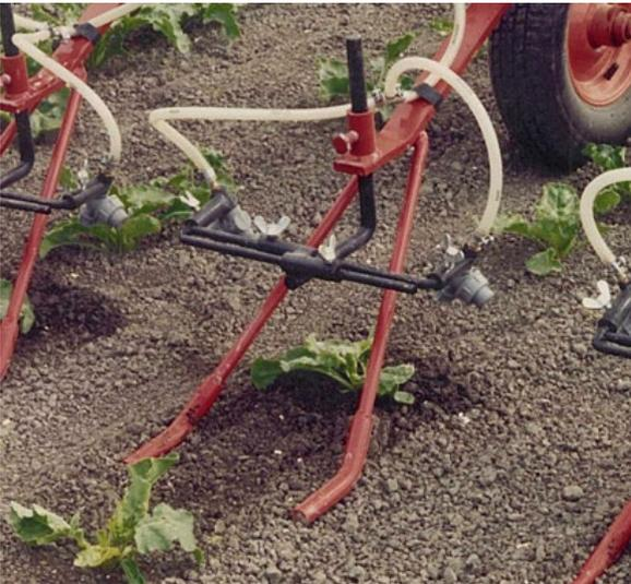
**Figure 7A** Sprayer for row specific application
