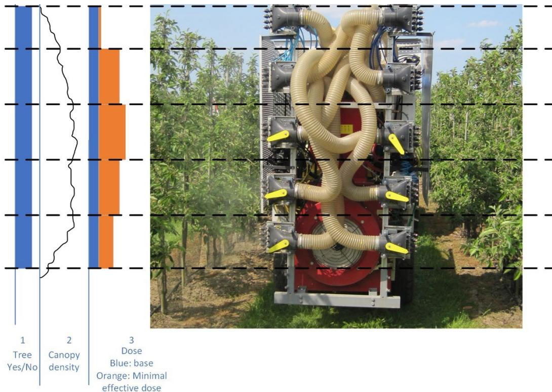
**Figure 5** Technical representation of precision-application *precision-spraying in tree fruit production*
