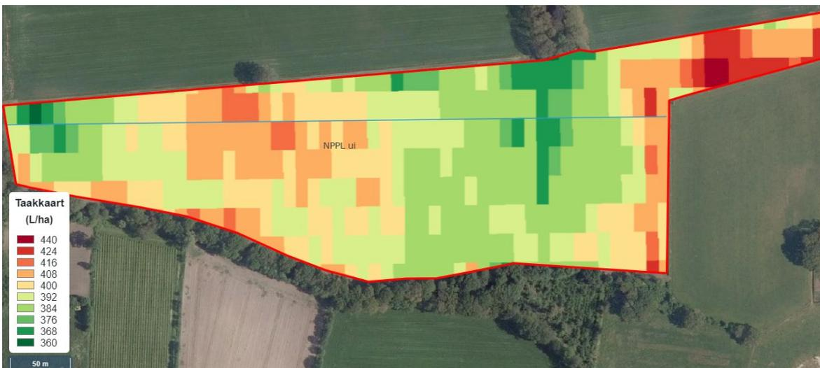
**Figure 2C** Task-map displaying spray volume adjusted to working width of the sprayer, in litres tank-mix per ha
