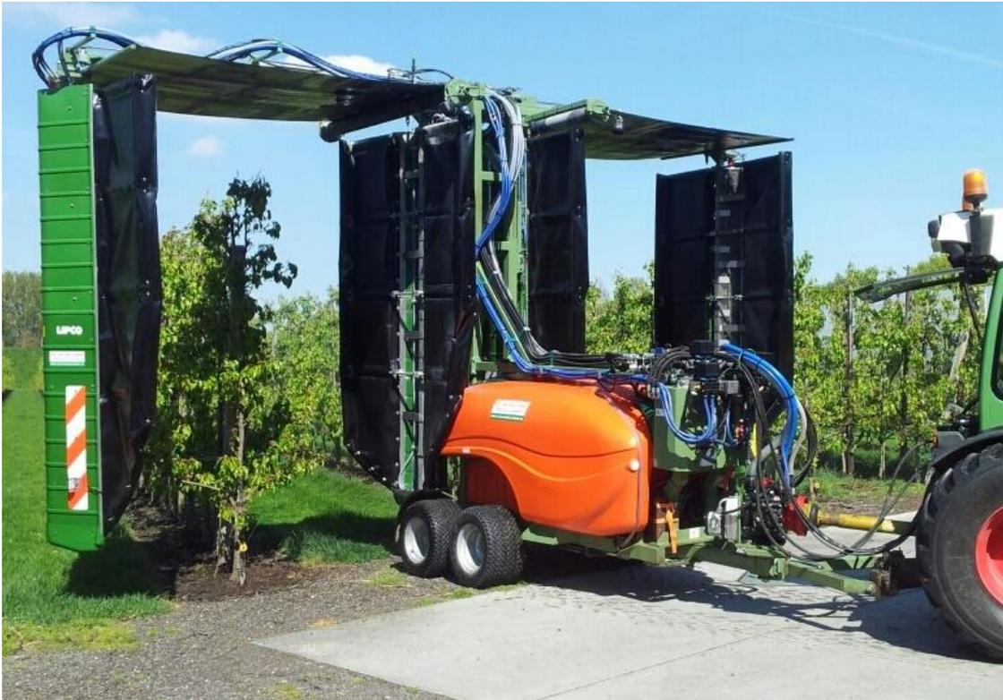
**Figure 9** Two row tunnel-sprayer with recirculation-system
