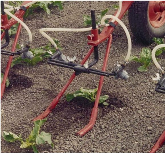
**Figure 7A** Sprayer for row specific application
