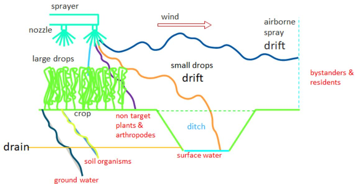
**Figure 10** Schematic representation of exposure-routes and protection goals during the application of plant protection products in open field production. Position of the spray nozzle (off center nozzle) is dependent on the crop.
