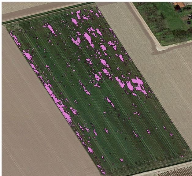
**Figure 4** Task-map for spot spraying weed control of sow thistle
