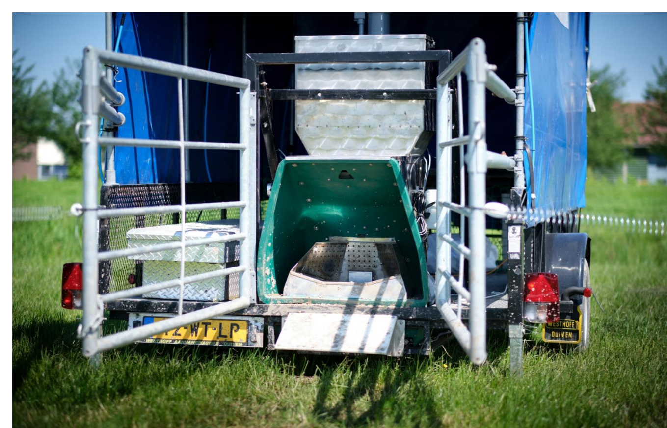
Figure 1. A GreenFeed unit can record CH 4 and CO 2 production (g/day) in a pasture or a barn.
