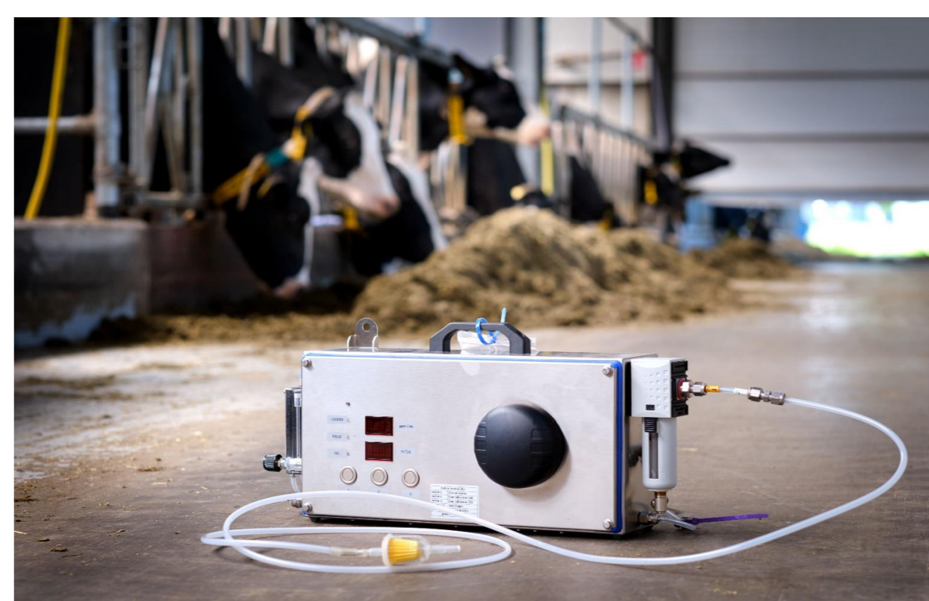
Figure 2. The "sniffer" records CH 4 and CO 2 concentrations (ppm) in the feed bin of milking robots.
