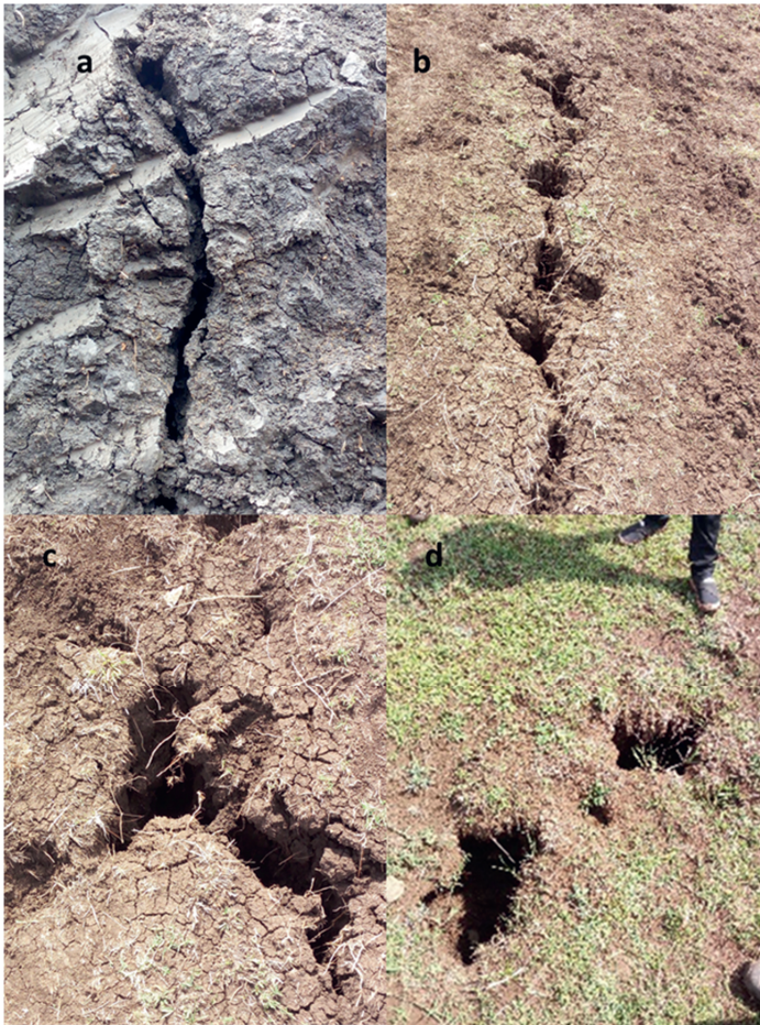
Figure 7.1 (a) is a soil crack observed in the soil profile. (b) and (c) shows photos of the cracks before the onset of the rainy season each depicting straight shaped crack, and cracks intersecting each other and become wider. Figure d shows cases where cracks grow into soil pipes.
