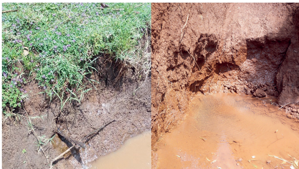
Figure 7.2 Soil pipe evidence in the gully bank that discharges water to the channel
