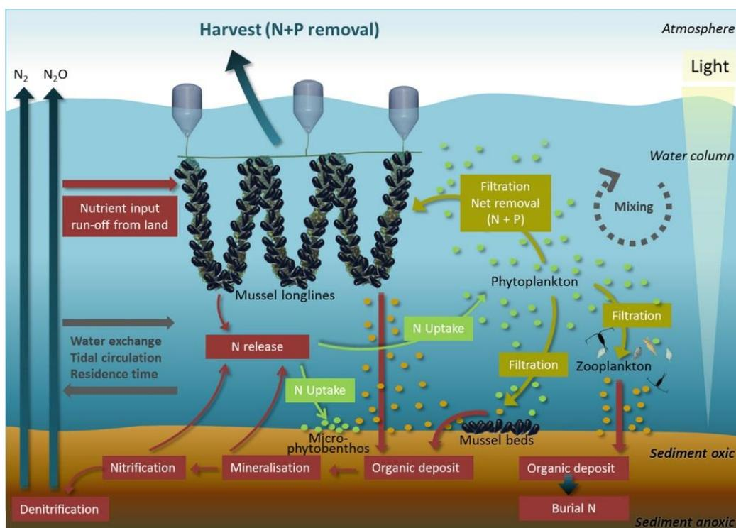
Figure 2. nutrient cycle of seaweed and bivalve production.
