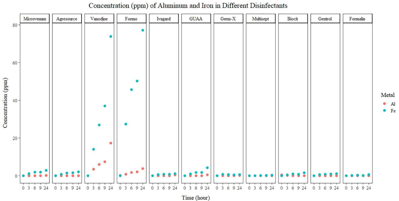
**Fig. 5.** Corrosiveness of disinfectants toward aluminum (Al) and iron (Fe) after 3-, 6-, 9-, and 24-h exposure to 11 disinfectants (1× dilutions) and expressed as concentrations of Al and Fe ions in parts per million (ppm). All experiments were conducted twice and the means for both experiments are shown as dots.
