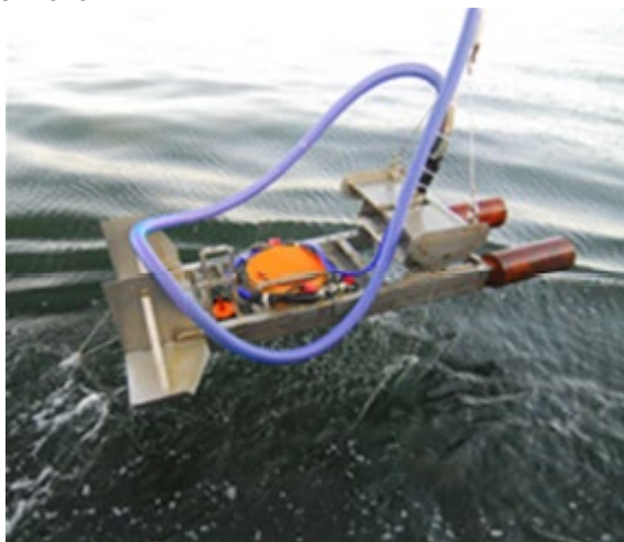
Figure 5.2 Towed body with 38 and 200kHz transducers. The purple hose protects the electrical cable that is connected to the EK80 in the steering house.
