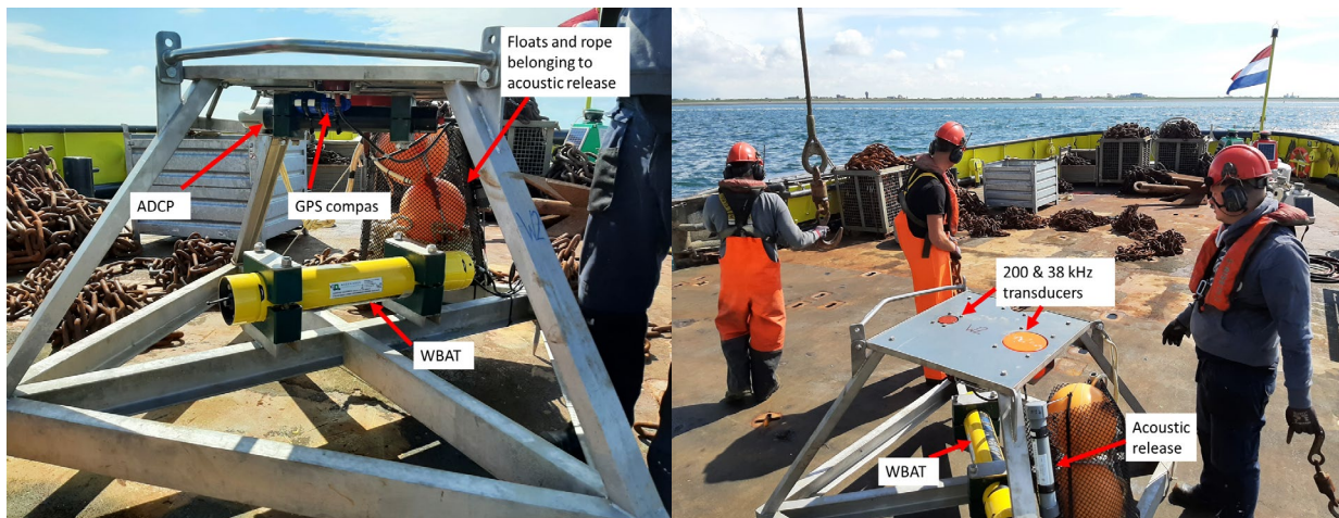
Figure 5.8 RVS frame with Wbat, as deployed in the Marsdiep.
