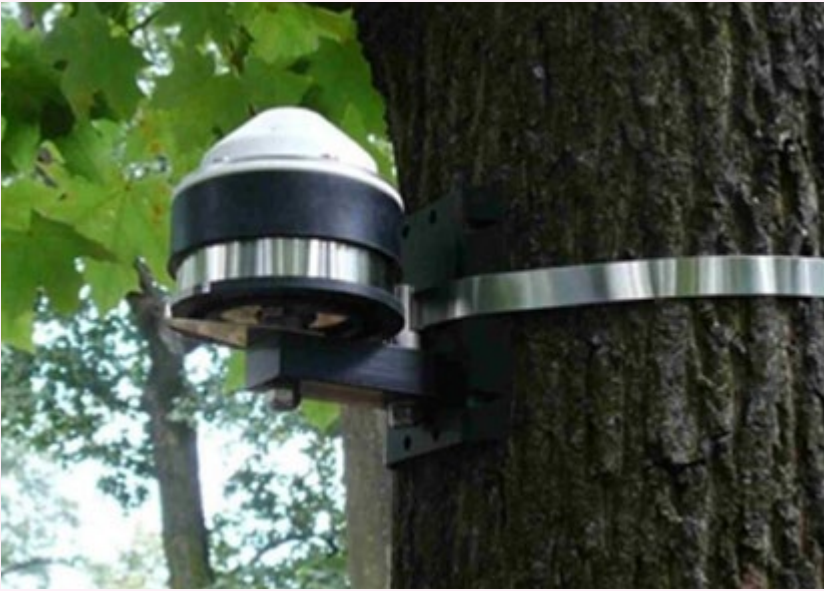
Dendrometers accurately record changes in trunk diameter • Photo Bas Lerink
