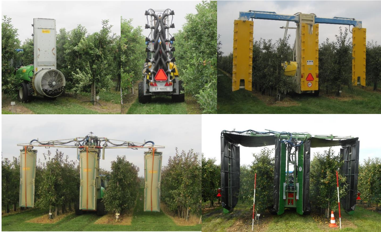
Fig. 2. Sprayers used for assessing spray deposition in the full leaf stage of the apple trees: Munckhof cross-flow (top left), H.S.S. cross-flow (top centre), KWH multiple-row cross-flow (top right), Lochmann 2-row tunnel (bottom right), Munckhof multiple-row cross-flow (bottom left).
