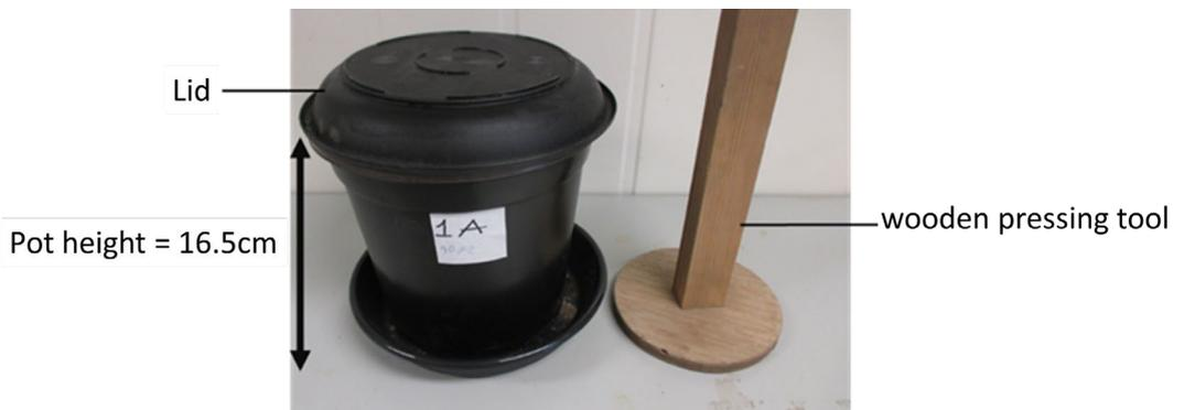
**Figure S4.1:** Pot and wooden pressing tool.
