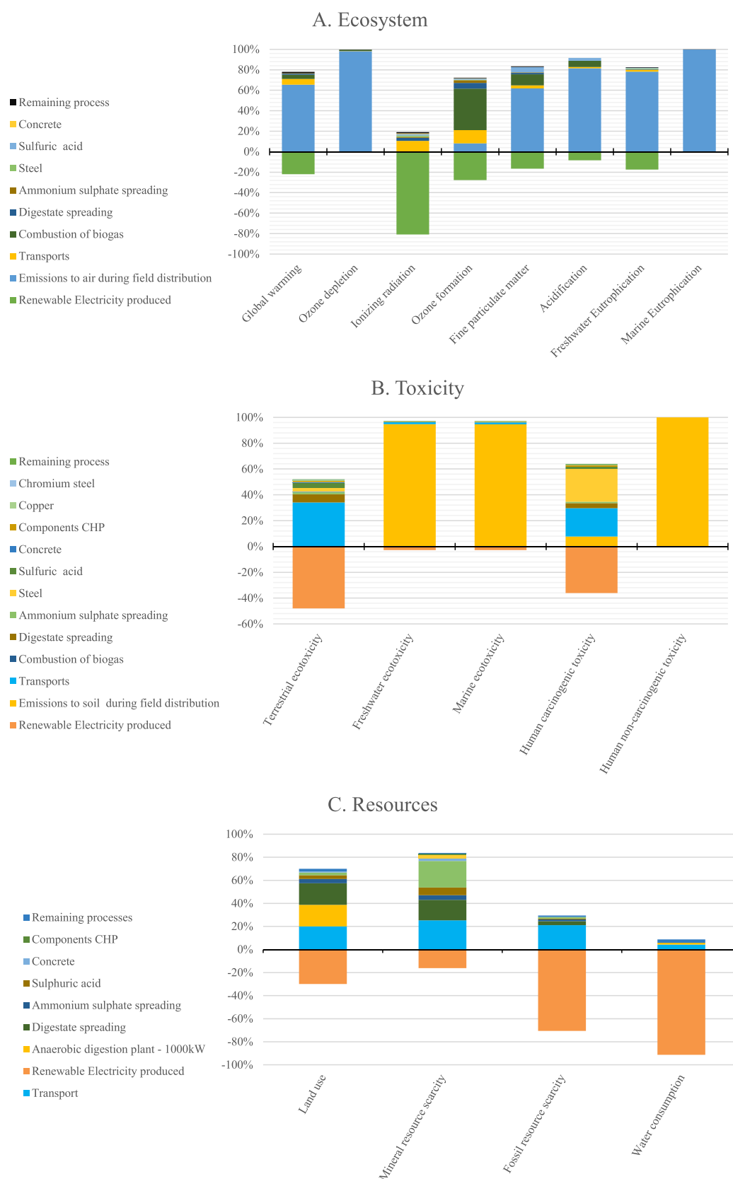
Figure 3. Process contribution to the impact categories of the Scenario RF, focusing on the ecosystem (a), toxicity (b), and resources (c). Impact assessments were calculated according to the ReCiPe 2016 midpoint (H) V 1.03 method and data reported as percent of the total impact.
