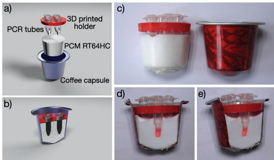
**Figure 1.** a,b) 3D render of the T-Cup showing its components: an aluminum coffee capsule, few grams of phase change material (RT64HC), a 3D printed holder for the LAMP vials, and the PCR tubes with the reagents in them. c) Picture of the T-Cup and d,e) picture of the cross-section, highlighting the distance between the bottom of the vial and the aluminum capsule.
