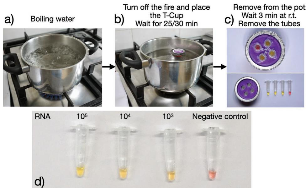
**Figure 3.** Procedure for the T-Cup LAMP test. Top: a) turn on the fire and wait for the water to boil. b) Turn the heating off, put the T-Cup inside and wait for 25/30 min. c) Remove the T-Cup from the water, let it cool down and remove the vials. d) Example of successful amplification and detection of SARS-CoV-2 using the T-Cup.
