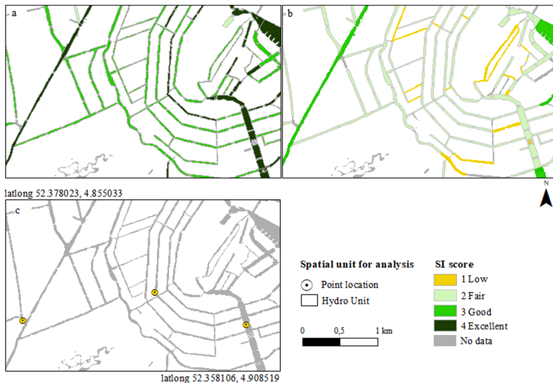
Fig. 3. Application of the SIs provides spatial information about the suitability of urban surface water for individual use functions in a comparable way. This is illustrated by the SI scores for TEE (a), Transport (b) and Recreation (c) for part of the city centre of Amsterdam. See Supplementary material Fig. S1 for full maps and Supplementary material DS1 for all data per HU or point location.
