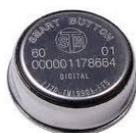
**Photo 2.** Ibutton device for temperature recording
