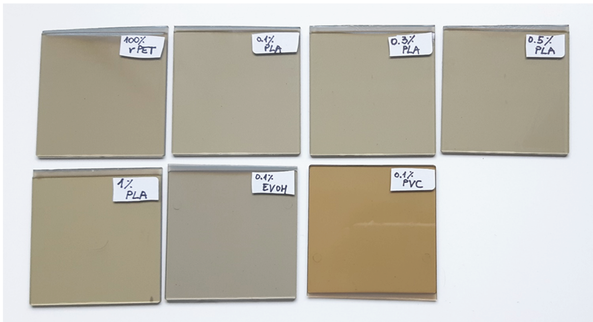
FIGURE 2 Photo of the 5 \times 5 \times 0.2 cm plaques of the recycled PET with various impurities, clearly showing the colour
