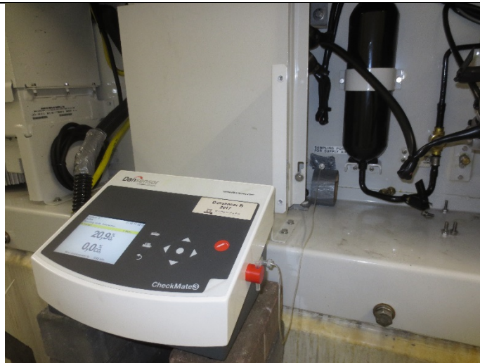
Fig. 16, Dansensor sampling through the unit's sampling port for supply air.
