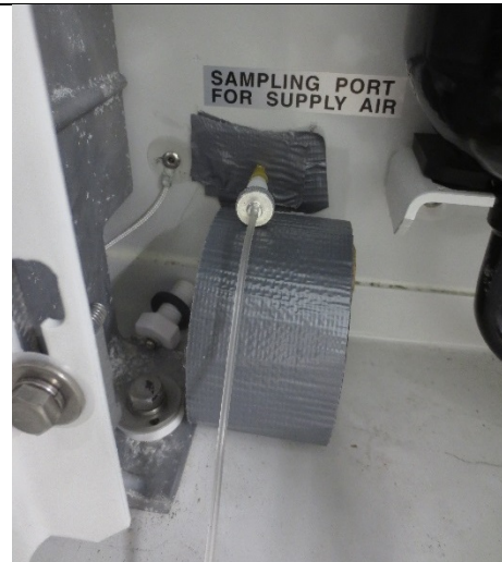
Fig. 17, Dansensor sampling through the unit's sampling port for supply air.
