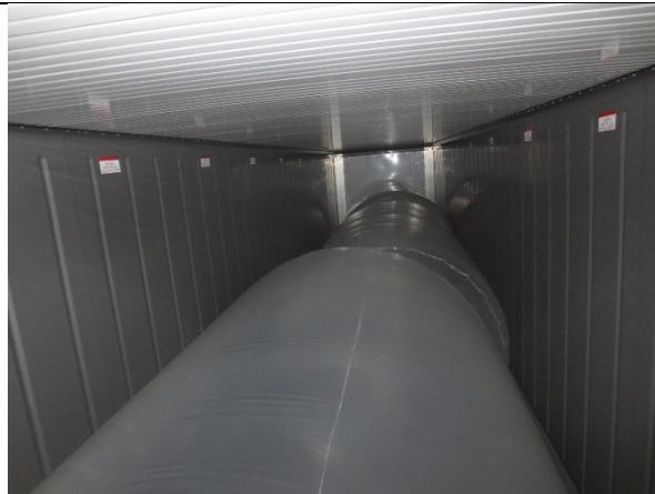
Fig. 22, three balloons of 10 m 3 each, observed at start and end of active system test.
