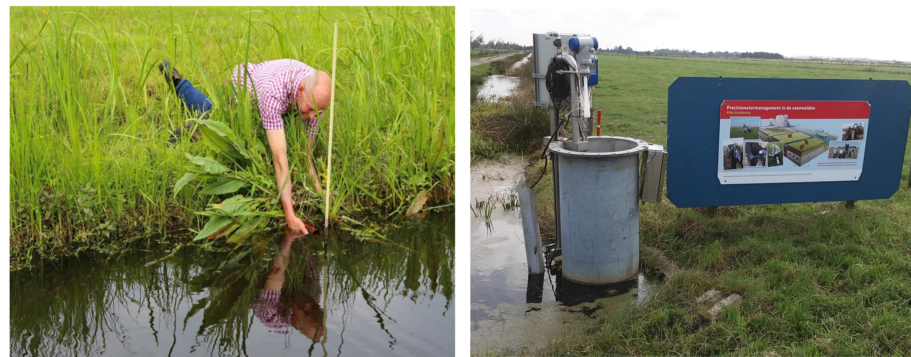
Figure 1. Left: ditch connected submerged drains. Right: water reservoir with pump and sonic reservoir water level measurement of pump-controlled submerged drains on experimental farm KTC Zegveld. The submerged drains are connected to the reservoir via a collector drain.
