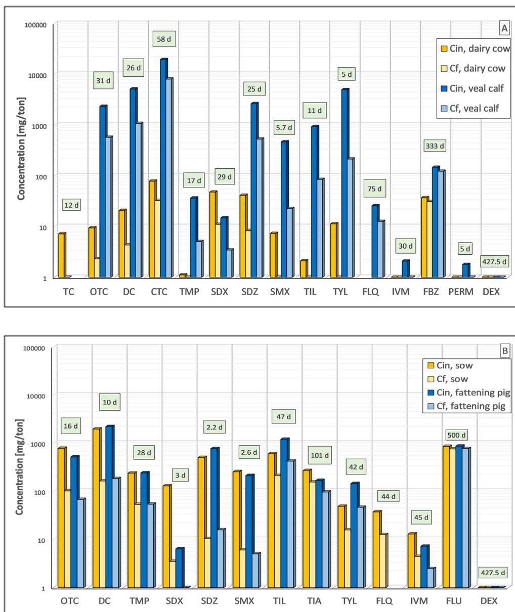
Fig. 4. Concentrations of VPs in slurry manure prior to storage (Cin) and after 6 months of storage (Cf) (log scale), including substance half-life in the storage (DT50 in days) displayed in the green text box. (A) In cattle sector for 15 different VPs. (B) In pig sector for 13 VPs. Cin is calculated with Eq. (1) and Cf with Eq. (3). Quantities of produced slurry manure (P) were estimated as 28 (dairy cow), 3.5 (veal calf), 4.5 (sow) and 1 (fattening pig) ton/animal per year.
