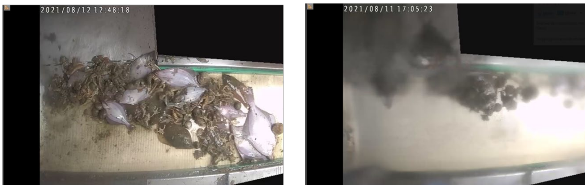
Figure 9. Fishers need to conform to the operational practices required on board to facilitate the success of EM, this includes cleaning lenses. Figure shows video shot from the same camera clean, useful data (left panel), and murky, useless data (right panel).
