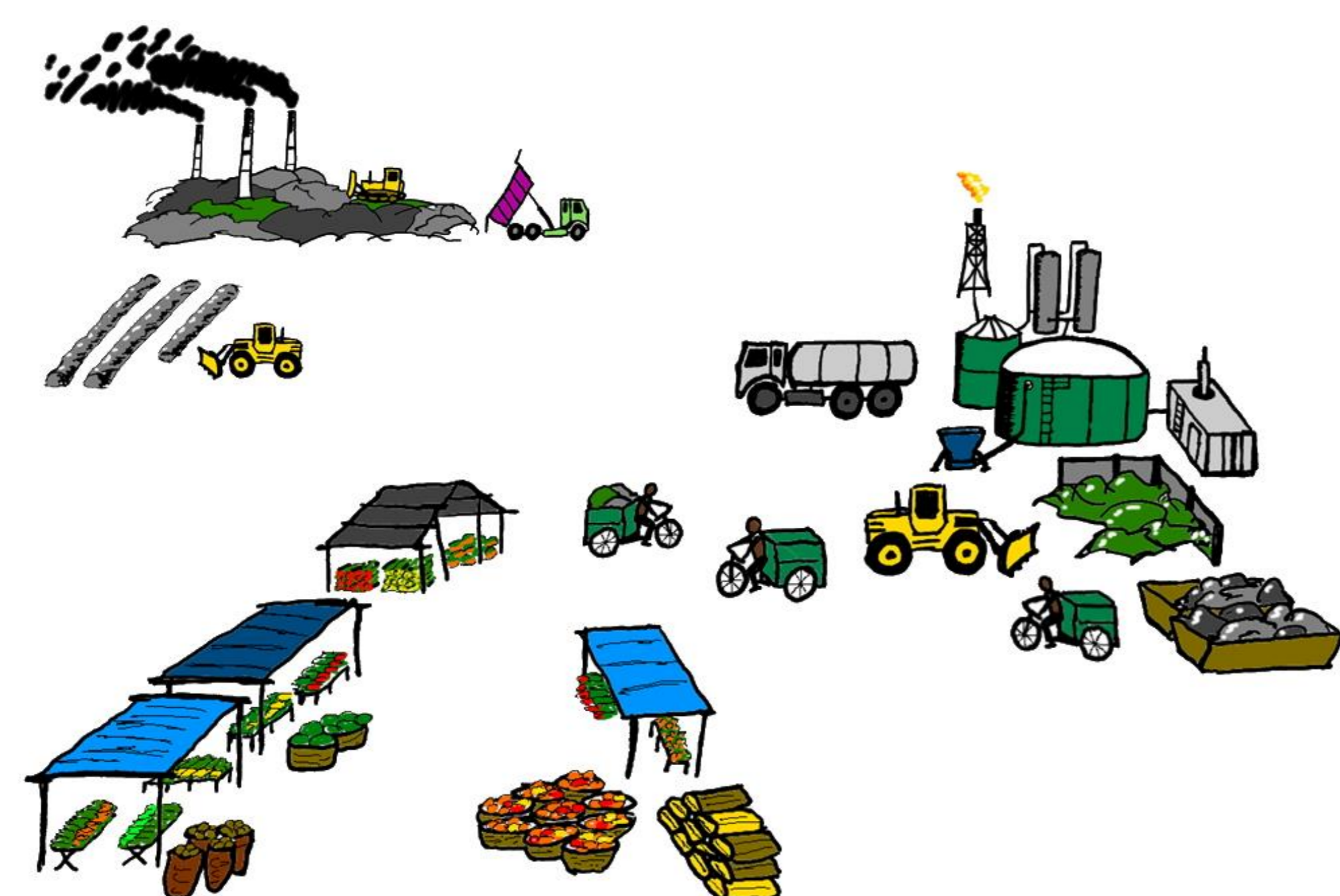
Figure 2. Anaerobic digestion of biodegradable waste. The secondary transfer station is partly replaced with an anaerobic digester, transport by trucks and landfilling are reduced, the solid fraction of the digestate is composted.
