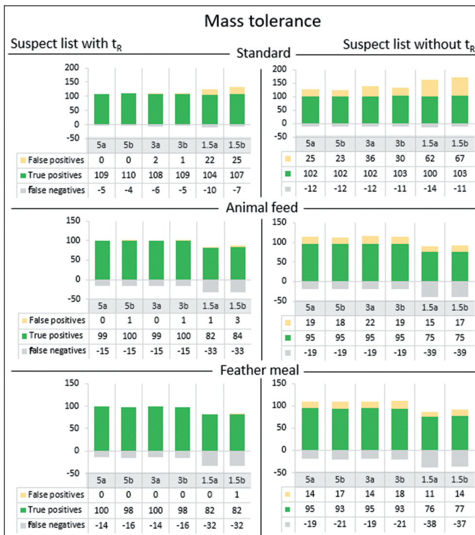
Figure 3. The effect of the mass tolerance (resolution = 140,000) set to 5, 3 or 1.5 ppm (in duplicate (a and b)) on the number of false positives, true positives and false negatives (expressed as a negative number in this bar graph) found in the standard mix solution, fortified animal feed and feather meal using a suspect list with and without retention times ( t_R ). The total number of substances in the standard mix solution is 114.
