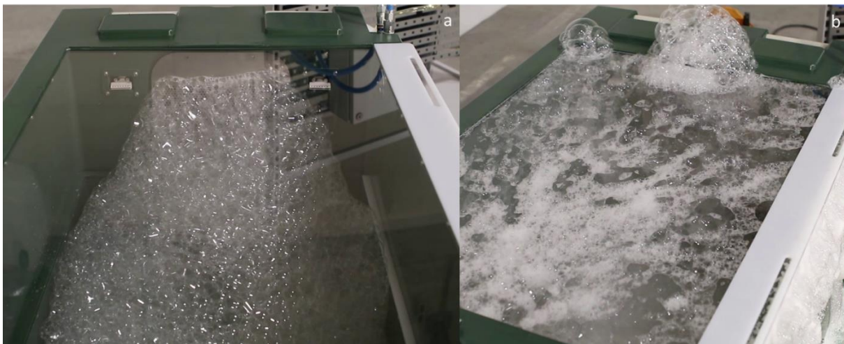
Figure 3.2.2 Foam system for piglets (© HEFT AB); after filling the box with nitrogen-filled foam (a), the foam is destroyed by the influx of nitrogen to allow a view of the inside of the box (animal area) and to remove air pockets (b).
