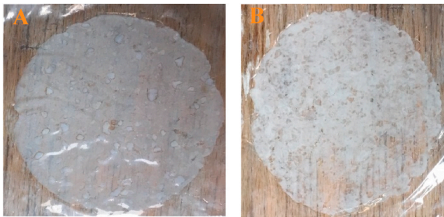
Fig. 7. Images of films prepared from dispersions originating from broiler breeder skins (A) and from fast growing broiler chickens (B) precipitated with 24% NaCl. The figure shows the resulting semi transparent film (image A), and opaque (B). Note: an opaque appearance is associated with a salt-precipitated dispersion forming a strong film.
