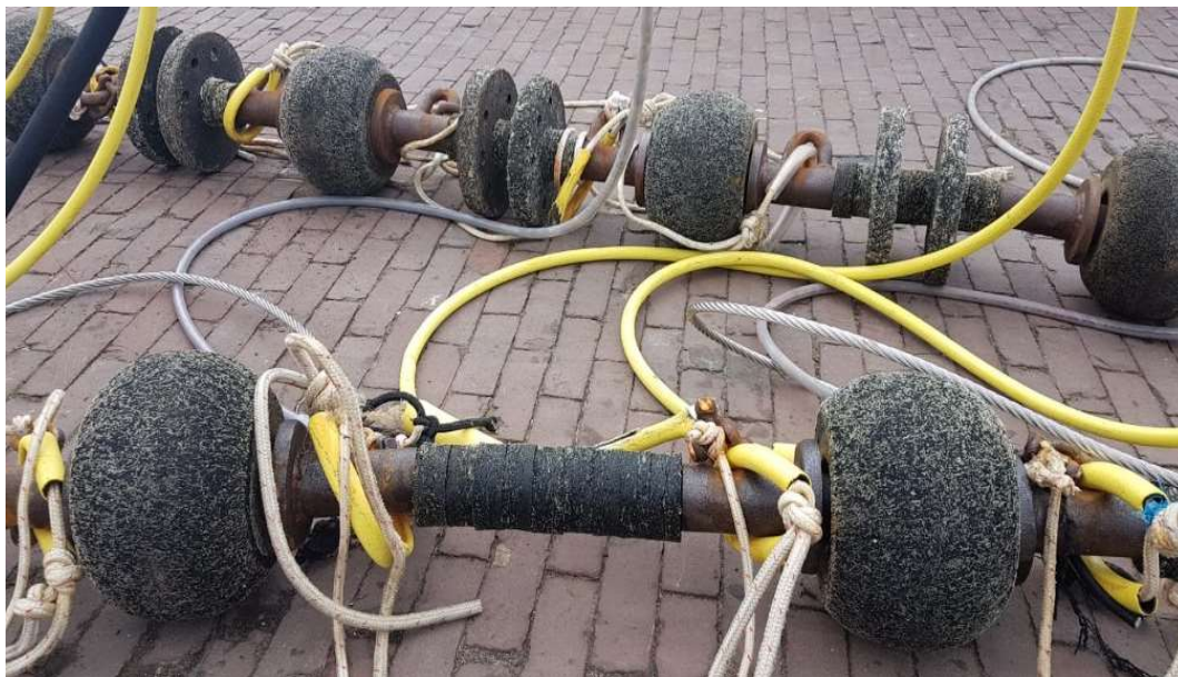
Figure 17: Close up of two bobbins in the standard straight bobbin rope configuration as obliged for pulse trawlers in the Netherlands (front) and the new bobbin rope with two additional rubber discs between the bobbins (back).
