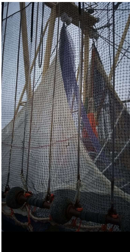
Figure 22: Sieve mat in the nets of the ST24.
