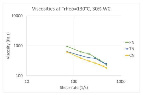
Different starch types result in different viscosity of the formulation!
