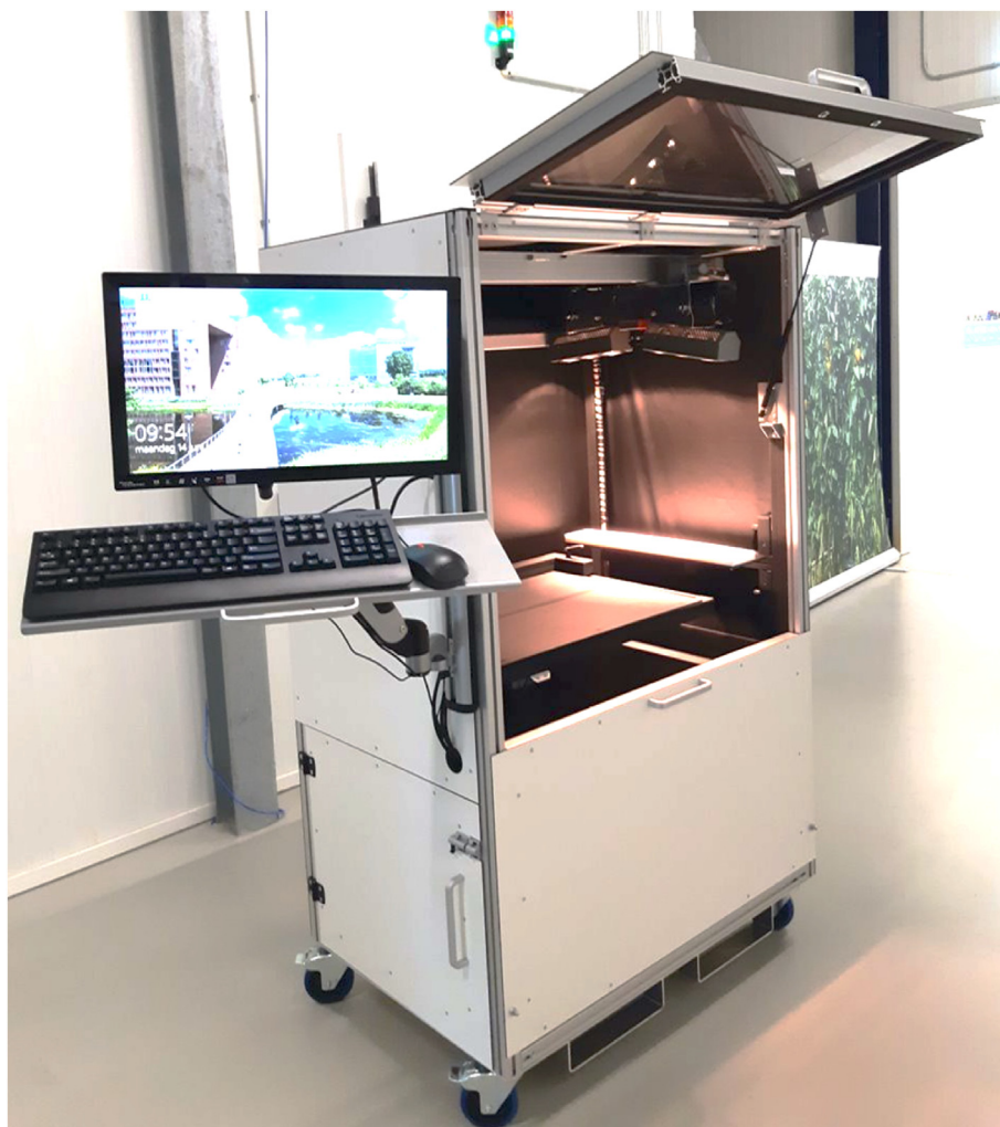
Fig. 1. The all-in-one spectral imaging setup used for data acquisition. This all-in-one [37] setup provides a fully automated approach to spectral imaging and the final output of the setup is the raw reflectance data.
