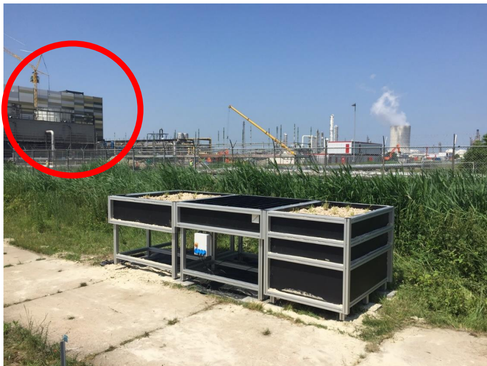
Fig. S7-1. Pilot-scale hybrid constructed wetlands, located close to the cooling tower (red circle). Cooling tower water flows from right to left vertical subsurface-flow constructed wetland → surface flow constructed wetland → horizontal subsurface flow constructed wetland.
