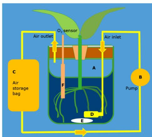
Figure 1. Closed system with an air-tight vessel containing nutrient solution, plant roots and air (A), a peristaltic pump (B) and an air storage bag (C) with inside the vessel an air stone (D), a stirrer (E) and an O<sub>2</sub> sensor (F).
