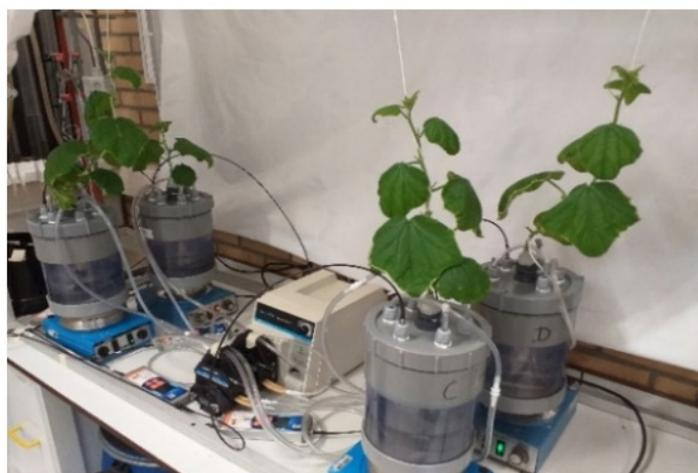
Figure 4. Four closed systems as Figure 1 with four cucumber plants. The O<sub>2</sub> sensor is inserted in the nutrient solution of each vessel.
