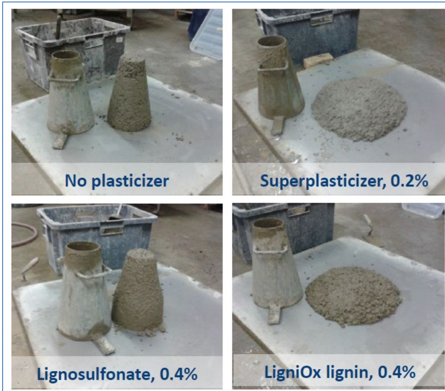
Figure 3. 5 Performance of the lignin-based superplasticizer LignOX
