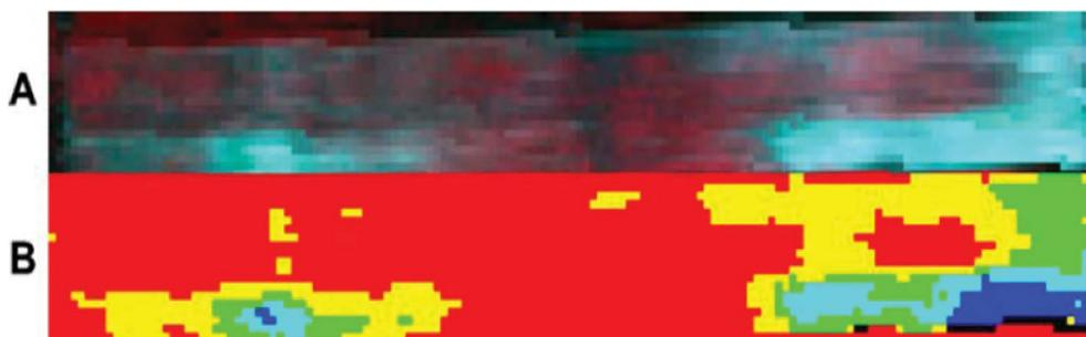
**Fig. 60.2.** AISA hyperspectral false colour infrared picture at GS 31 and digital map of *Heterodera schachtii* damage clustering. **(A)** Infrared photograph; **(B)** digitalized computer map with colours correlated with final nematode (*Pf*) densities (Hillnhütter *et al.*, 2011). Author's own figure.
