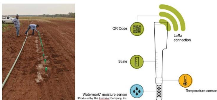
**Fig. 60.1.** Soil sensors (Valenco GmbH, Switzerland) for monitoring temperature and moisture relationships on nematode population development in microplots. Figure courtesy of M. Goll, Syngenta, Switzerland.
