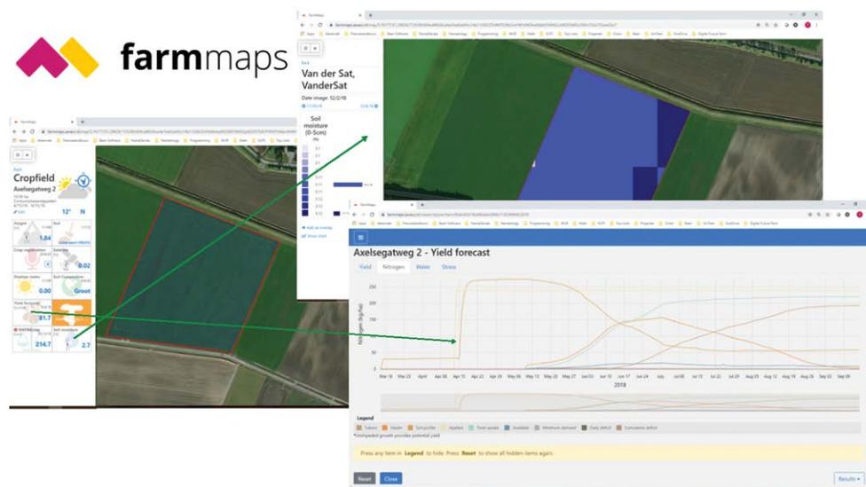
**Fig. 60.5.** An impression of the dashboard of FarmMaps. All information of a field can be reached via the widgets. In this figure soil moisture and the yield forecast of potato are highlighted. Figure courtesy of Wageningen University & Research, Field Crops.
